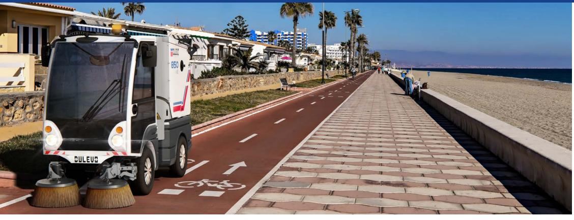
The innovative, modular structure, without the use of electronics, the belt-driven components and the easily removable side-mounted water tanks, simplify the access to all important components for service and maintenance. An additional maintenance hatch below the driver's seat and the button window support easy daily interventions on the suction mouth and hose.
